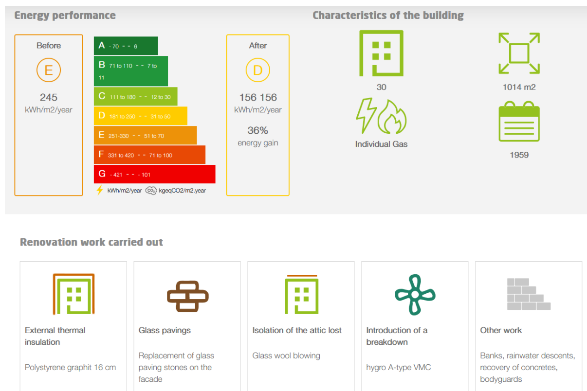
Figure 4. Results of renovation in Reims
